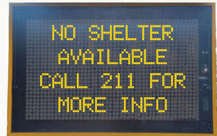
LA DOTD uses Variable Messaging Signs (VMSs) to send messages to drivers.
